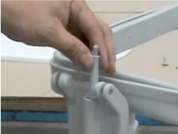
Step Six Insert soft closure mounting
