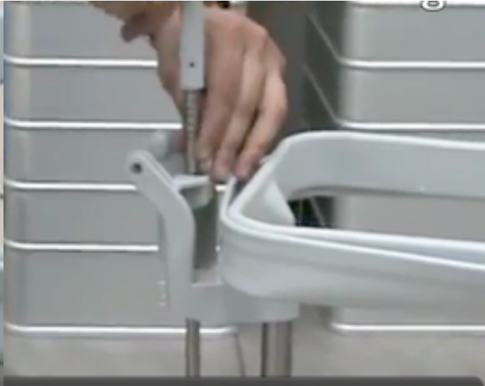
Step Seven Pedal tube mounting Insert spring in the tube Insert tube in the housing
