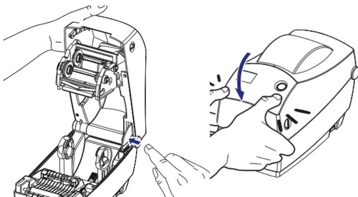
Roll the wheel on the left side core holder away from you to take up any slack in the ribbon. Close the top cover. Remember that you need to release the cover lock, lower the top cover, and press down until the latches snap into place..
