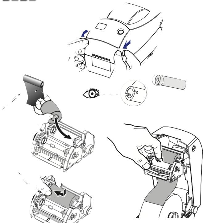
Now insert the core on the other end of the ink ribbon to the **Lower** set of core holders. Its very important that the notch cut out the the cardboard core lines up with the lugs on the left side core on both rolls
