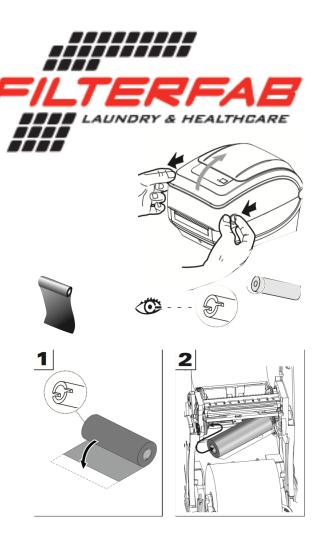
Now insert the core on the other end of the ink ribbon to the UPPER set of core holders.
