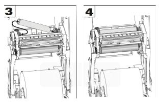
Its very important that the notches cut out of the cardboard core lines up with the lugs on the left side core holders
