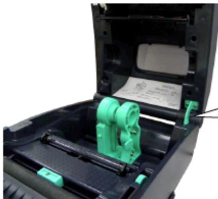
2. A top cover support at the rear of the printer will engage with lower inner cover to hold the printer top cover open.
