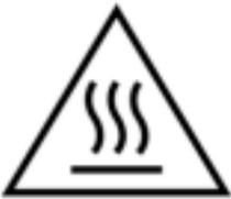
**Caution:** The printhead may be hot and could cause severe burns. Allow the printhead to cool.
