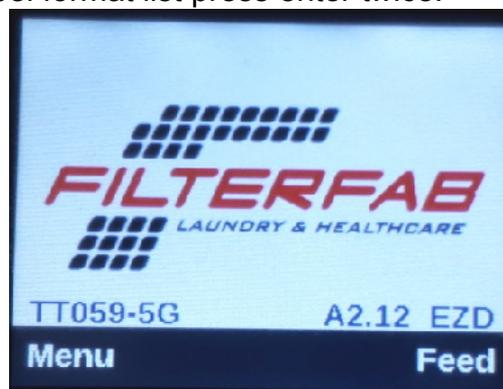
If the program exits to the main screen see above or any other issue just turn the power switch off and on the printer will restart and go into the label format menu.
